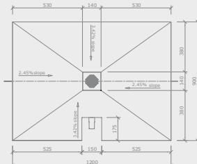
Fundo Plano, point drain, 1200 x 900 mm, short side connection
