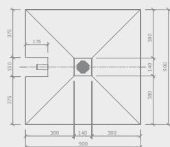
Fundo Plano, point drain, 1200 x 900 mm, long side connection
