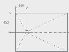
Drain position for 1800 x 900 mm
