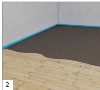
2 Apply tile adhesive to the wooden substrate.
